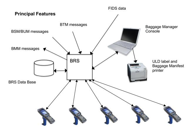
Baggage data is received from the airline DCS systems in the form of messages as defined in IATA RP1745, 1740, and 1800. These messages can be send to the BRS system via a type-b message link or via the Baggage message link.
